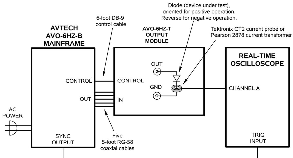
If a Tektronix CT2 current probe or Pearson 2878 current transformer is not available to measure the output current waveform, or the output pulses are too wide, a 1 Ohm resistor may be used to sense the current instead. However, noticeable ringing and
