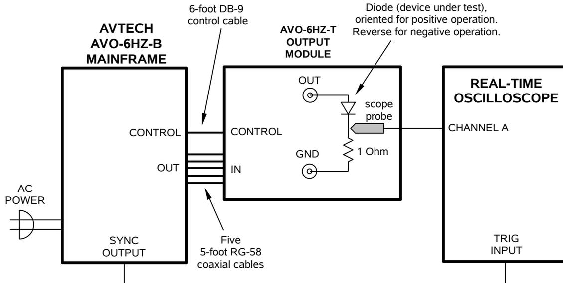
If the AVO-6HZ-B is operated at its maximum duty cycle, the worst-case power dissipation in the output module is  $(110V \times 10A \times 5\%) = 55$  Watts. The internal fan must have sufficient external ventilation to cool the module. The DB-9 control cable must be connected as shown above for the fan to operate.
