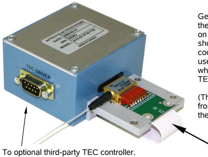
Gently slide the low-bandwidth slide-on socket onto the matching pins of the device under test. The slide-on socket is connected to the output module using a short length of flexible ribbon cable. The thermoelectric cooler and thermistor pins are made accessible to the user through the “TEC DRIVER” DB-9 connector, which will mate to cables from common third-party TEC controllers.
