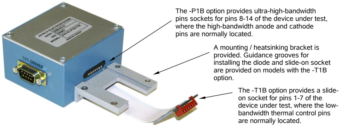
The diode is first installed by sliding pins 8-14 into the “P1B” pin sockets, as shown below:
