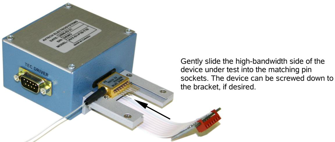
If present, the T1B slide-on socket assembly can then be slid onto pins 1-7, as shown below:
