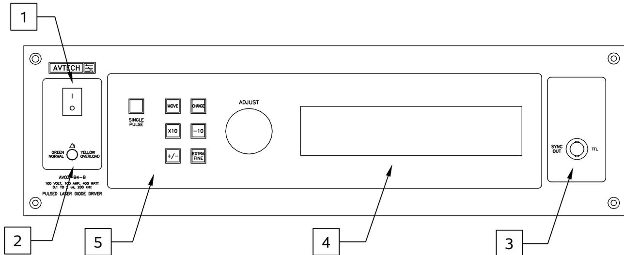
1. POWER Switch. This is the main power switch. When turning the instrument on, there is normally a delay of 10 seconds before anything is shown on the main display, as the internal operating system boots up.
