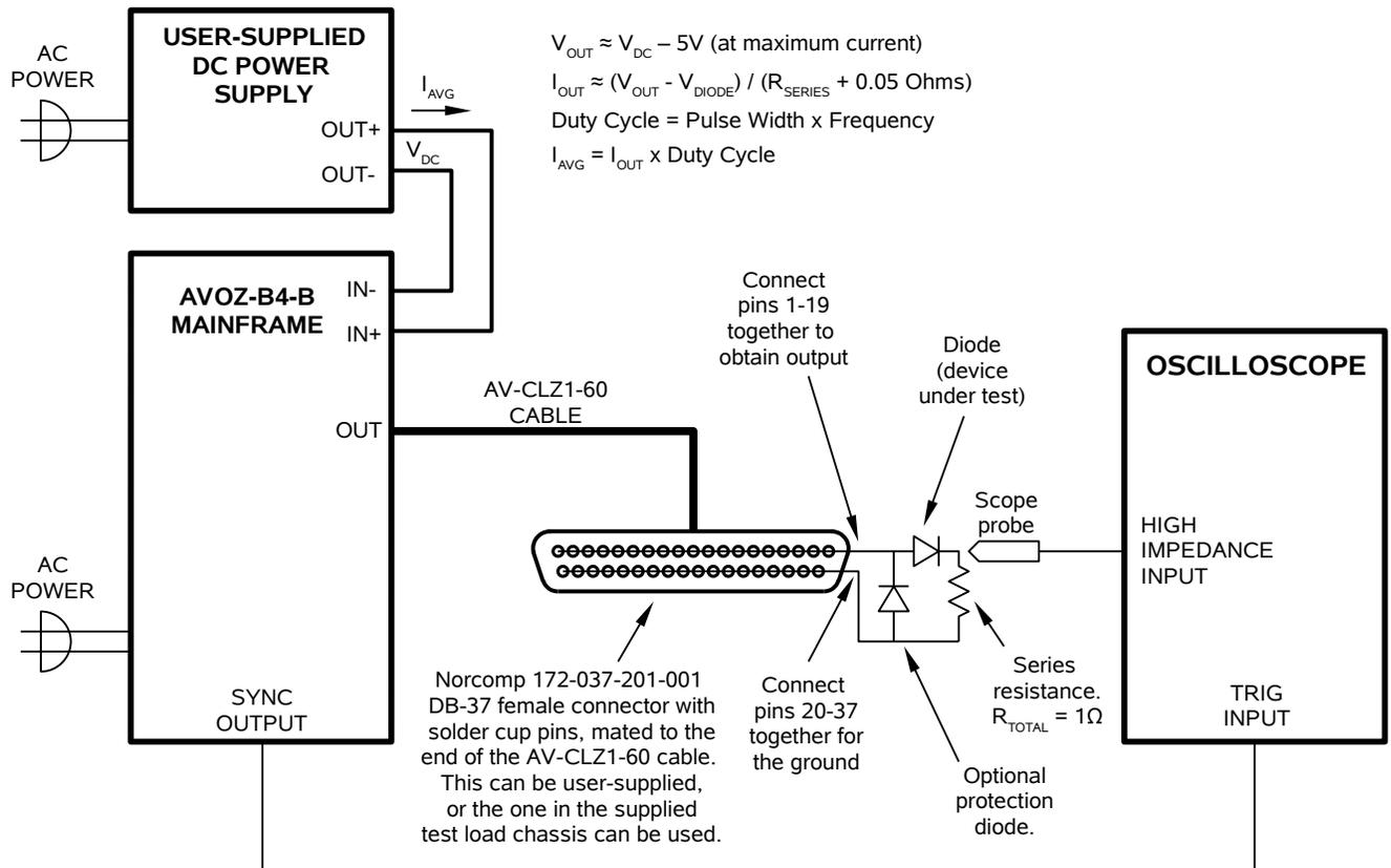
The loads can be connected to the pulse generator using the convenient AV-CLZ1-60 transmission line cable assembly, which has a 1Ω characteristic impedance ( $Z_0$ ), and is terminated with a DB-37 male connector. A sample low-power connectorized test load is provided for initial testing purposes.
