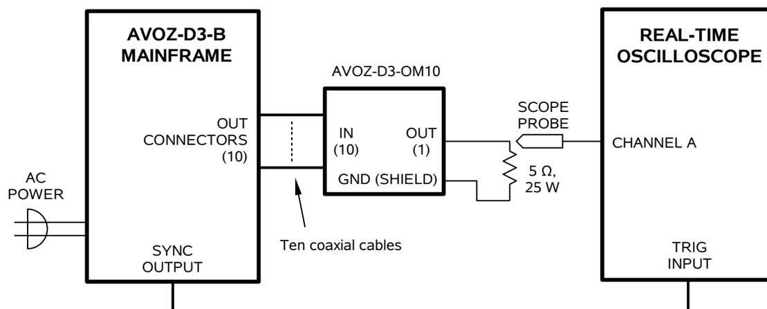
The output module is not needed if each output is driving its own load, as shown below:
