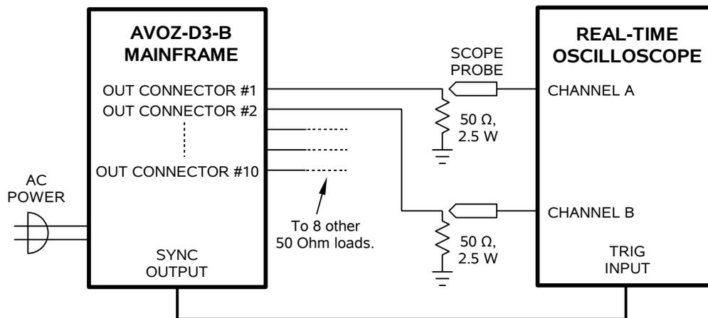
1. Connect a cable from the SYNC OUT connector to the TRIG input of an oscilloscope.
