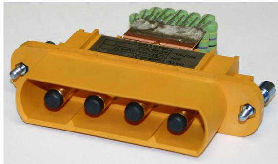
The user may use the provided resistance as-is, or disconnect one end to allow a diode load to be added in series with it, or remove the resistors entirely and connect to a different load as needed.
