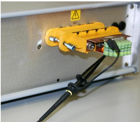
2. Set the oscilloscope to trigger externally with the vertical setting at 50 Volts/div and the horizontal setting at 1 us/div. Be sure that your oscilloscope and probe setup can handle the maximum amplitude of 100V.
