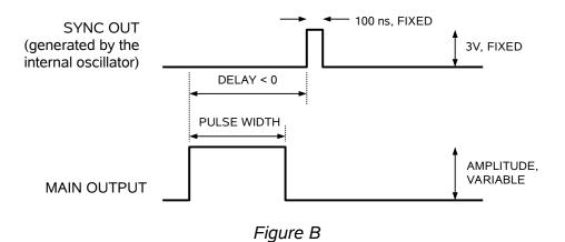
The next figure illustrates the relationship between the signal when an external TTL-level trigger is used:
