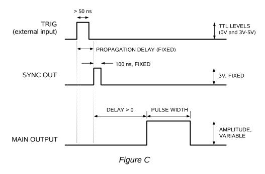
As before, if the delay is negative, the order of the SYNC and OUT pulses is reversed.
