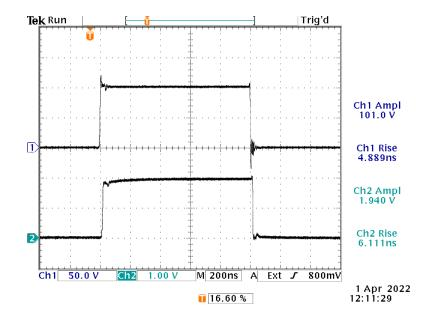
Top: +100V pulse, internally (before  $Z_{OUT}$ ) Bottom: resulting +2A current, measured with a CT2 current probe (1V/A).
