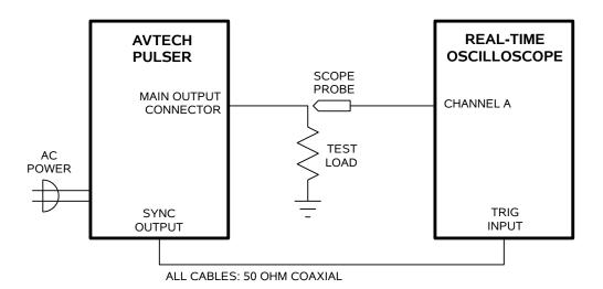
1. Connect a cable from the SYNC OUT connector to the TRIG input of an oscilloscope. Connect a 50W (or higher)  $50\Omega$  load to the OUT connector and place the scope probe across this load. The load resistor <u>must</u> have a voltage rating of at least 250V. The power dissipated in the resistor is given by
