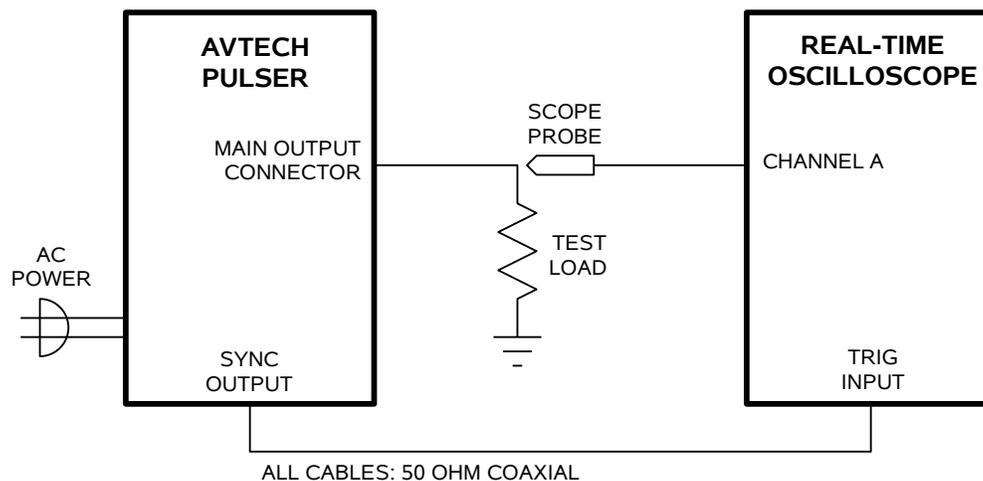
1. Connect a cable from the SYNC OUT connector to the TRIG input of an oscilloscope. Connect a 50Ω (or higher) load to the OUT connector and place the scope probe across this load. The load resistor must have a voltage rating of at least 500V. The power dissipated in the resistor is given by
