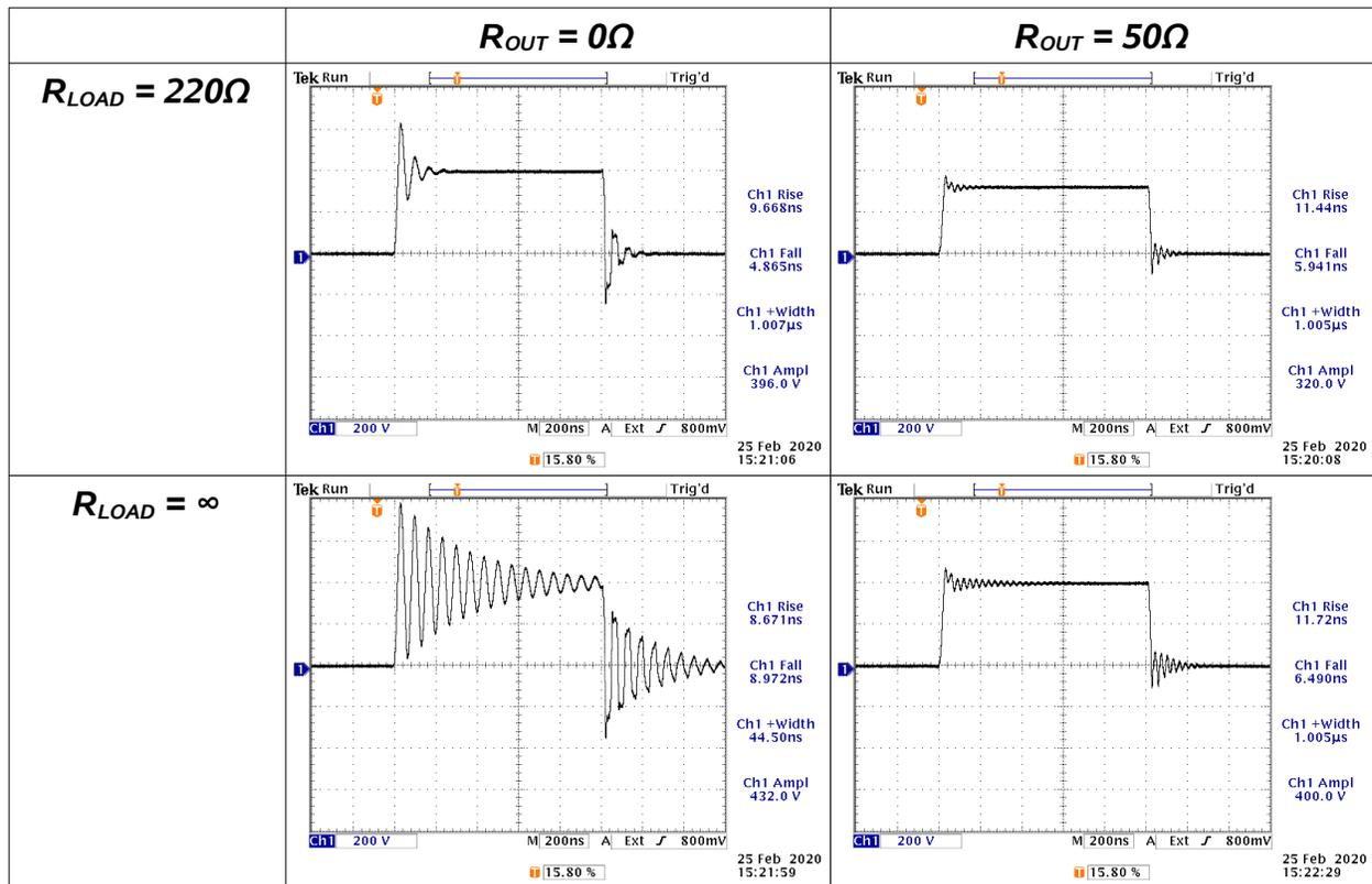
It should be observed that maximum voltages are obtained when  $R_{OUT} = 0\Omega$ , but transmission line reflections are minimized with  $R_{OUT} = 50\Omega$ . Also, regardless of the value of  $R_{OUT}$ , reflections and ringing are minimized when  $R_{LOAD} = 50\Omega$ .
