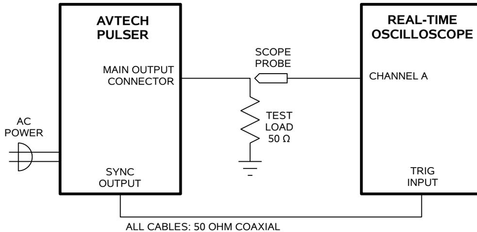
*BASIC TEST ARRANGEMENT, WITH A REAL-TIME OSCILLOSCOPE*
