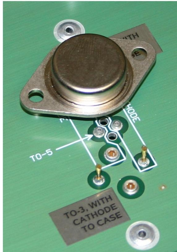
Only one of the two pins on the TO-3 package is electrically connected in this jig. This allows testing of dual-diode TO-3 packages, by rotating the package to isolate the desired diode.
