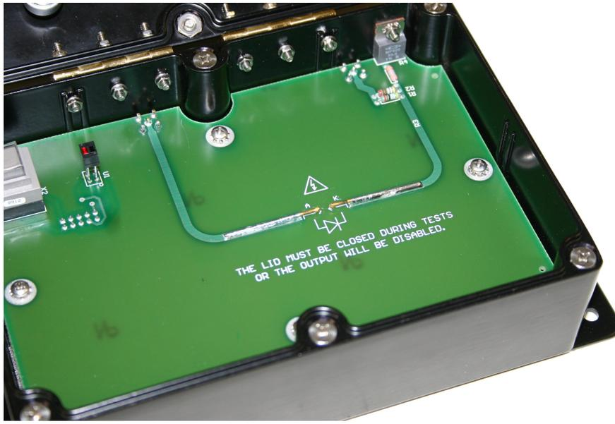
The next photo shows a MELF device installed between the two pins:
