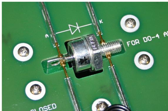
This diode produced the following results ( $t_{RR} = 2.595 \mu\text{s}$ ):
