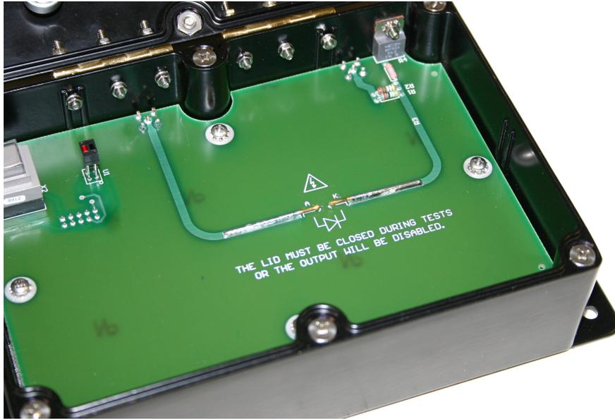
The next photo shows a MELF device installed between the two pins:
