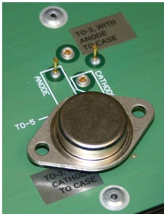
For the case-anode configuration, this layout is used:
