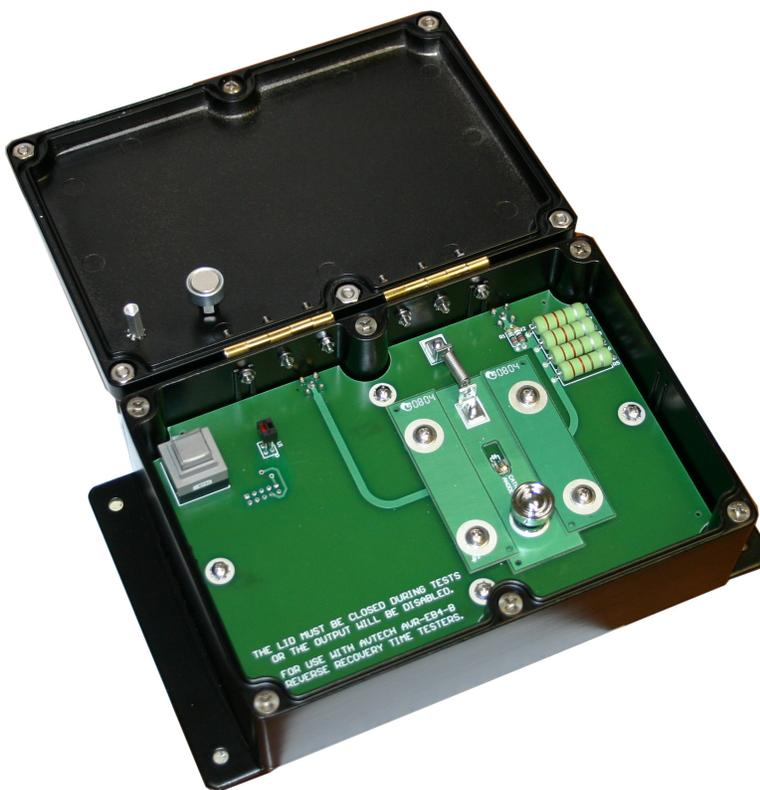
The DUT is installed by pulling back on the chrome knob, as shown below:
