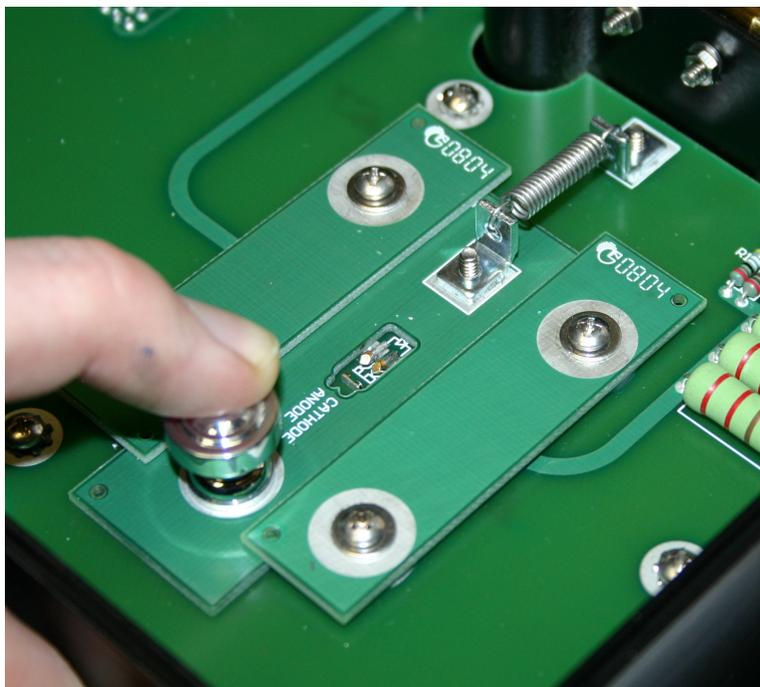
The DUT is then placed on its side in the area immediately in front of the two fixed probe points, as shown in the photo above. Then slowly release the chrome knob, allowing the spring-loaded PCB to push the DUT into position against the two probe points, as shown below. The PCB silk-screening shows the proper device positioning.
