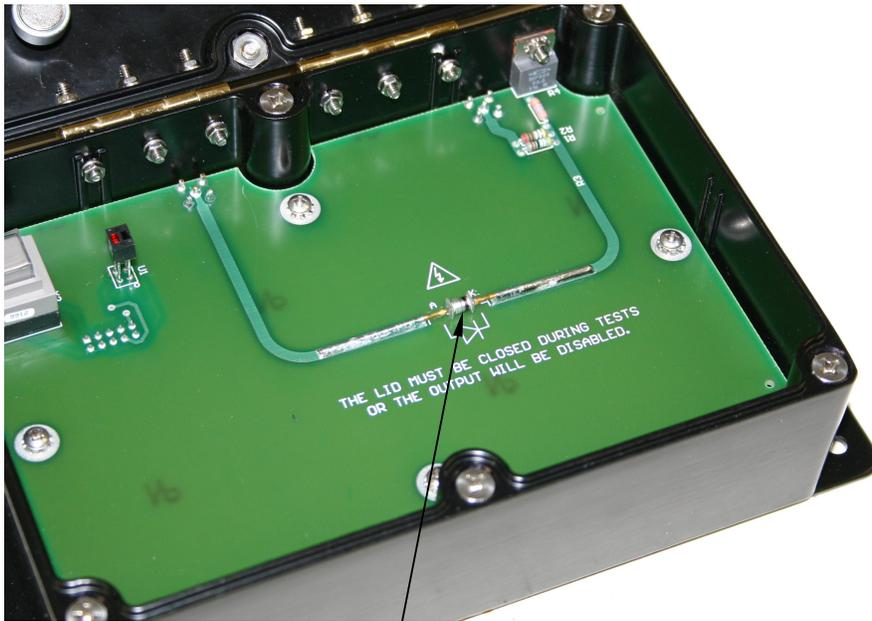
A MELF-packaged Device Under Test (DUT)
