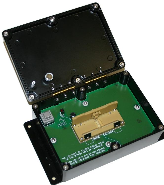
Insert a diode into one of the 4 “pockets”. The two gold contact pins are visible in each pocket; the device must be aligned with these pins. A DO-41 package is shown installed below:
