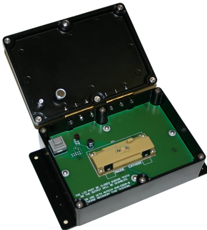
Then open the tan-colored DUT socket by flipping forward the two black latches on the front edge of it:
