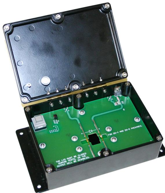
The photo below shows a reverse-polarity DO-4 diode (the Ruttonsha 12FLR60/F05) installed between the four spring-loaded contacts (two for the anode end, and two for the cathode end):
