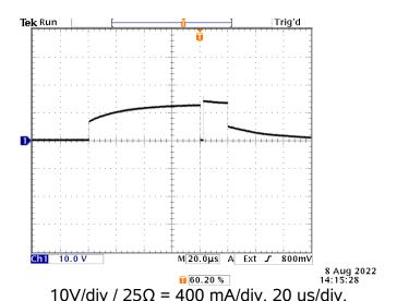
The SYNC pulse occurs shortly before the beginning of the reverse pulse. (The SYNC pulse is used to trigger the oscilloscope, and the location of the rising edge of the SYNC pulse is denoted by the orange "T" marker in the waveform above.) Changing the time scale to zoom in on the 2 us wide reverse pulse gives:
