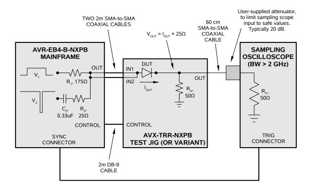
The total effective resistance of resistors  $R_A$  and  $R_C$  in the diagram above is  $50\Omega$  / 2 =  $25\Omega$ . Thus, the voltage at the jig output is simply given by:
