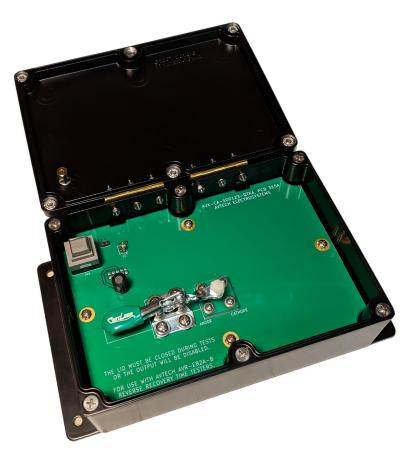
Raise the green lever on the left. This will raise the nylon screw over the DUT area on the right:
