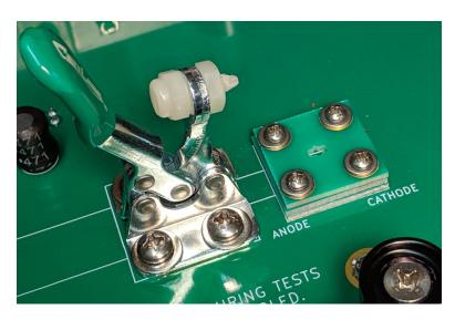
Using tweezers, position a DUT in the cavity of the raised circuit boards. Slots are provided for tweezer access. The DUT will rest on two spring pins, one contacting each DUT pad:
