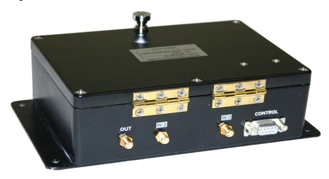
The IN 1 and IN 2 connectors are interchangeable. Both must be used, to connect to the two OUT connectors on the rear panel of the mainframe.
