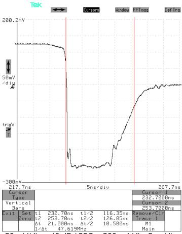
$50 \text{ mV/div} \times 40 \text{ dB} / 25\Omega = 200 \text{ mA/div}. 5 \text{ ns/div}.$
