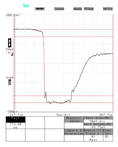
This waveform shows that the +0.5A to -1A switching time (10%-90%) is  $\sim$ 0.77 ns.
