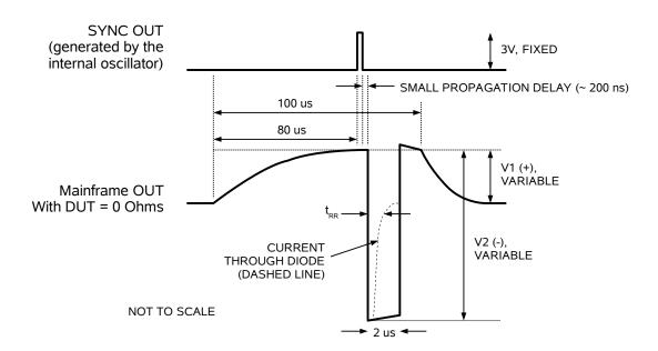
The forward-bias pulse  $(V_1)$  is approximately 100 us wide, and has a slow rise time (governed by the  $R_1 \times C_2$  time constant – see equivalent circuit in the "BASIC AMPLITUDE CONTROL" section for details about  $R_1$  and  $C_2$ .)
