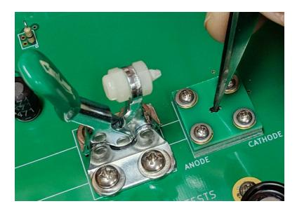
The cathode should be on the right. The anode should be on the left.
