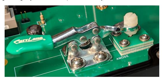
It is possible to use a screwdriver to adjust the positioning of the nylon screw. This will vary the maximum mechanical pressure applied to the DUT. The lever should snap into place when fully down, with a firm locking effect. It may be necessary to occasionally adjust this screw.
