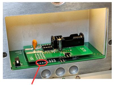
The left-most four GND2 pin sockets are used in the positive orientation.
