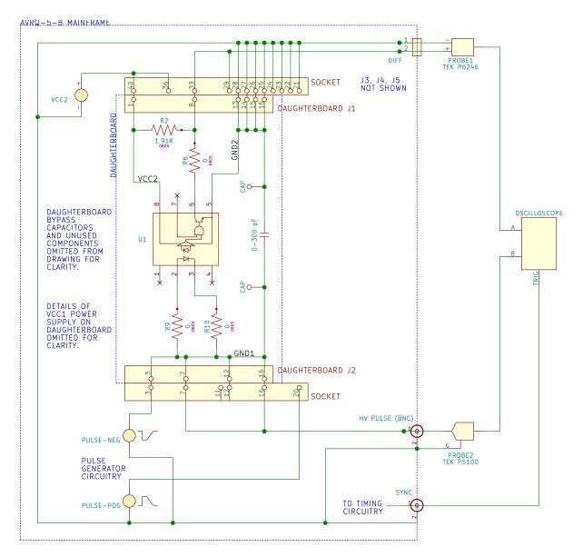
In the above drawing, an HCPL-2601 current-drive opto-coupler is installed on the daughterboard, and the daughterboard is configured to drive the opto-coupler input with zero current (by jumpering pins 2 and 3 to GND1). The daughterboard is positioned to connect the daughterboard to the negative pulse circuitry.
