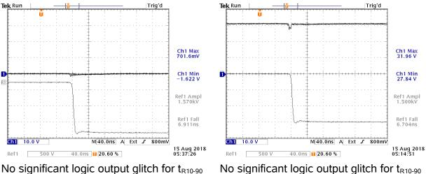
= 6.911 ns, so the CMTI exceeds 1.5 kV = 6.704 ns, so the CMTI exceeds 1.5 kV × (90%-10%) / 6.911 ns = 174 kV/us × (90%-10%) / 6.704 ns = 179 kV/us when  $I_F = 10$  mA.
