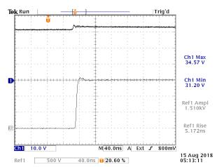
No significant logic output glitch for  $t_{R10-90}$  = 5.172 ns, so the CMTI exceeds 1.5 kV × (90%-10%) / 5.172 ns = 232 kV/us when  $I_F$  = 10 mA.
