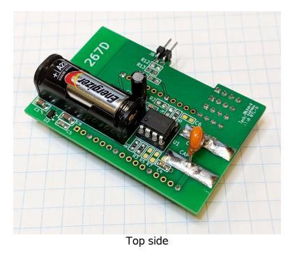
The actual daughterboard and DUT are shown below, configured for a 5V logic input:
