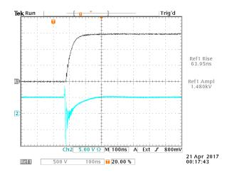
This shows an apparent 200 ns wide "glitch" on the logic output. In fact, the P6246 is saturating from the sharp initial inductive voltage spikes, and is taking 200 ns to recover.
