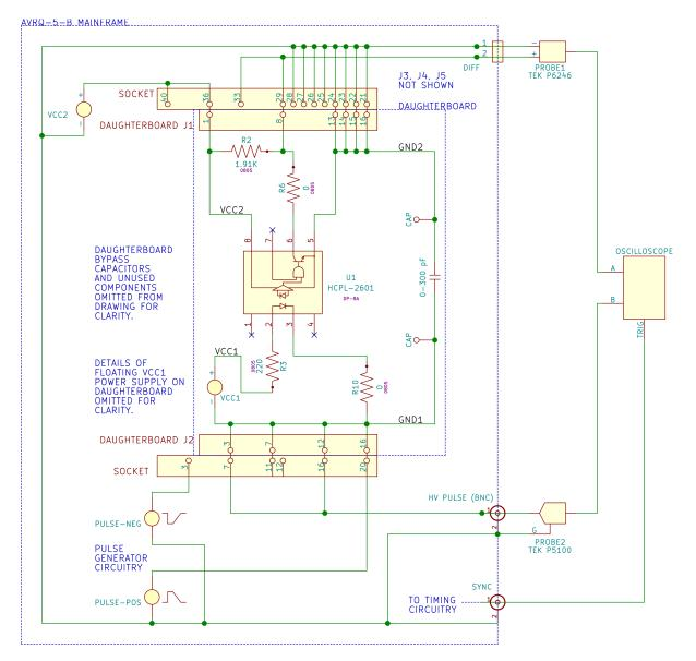
In the above drawing, an HCPL-2601 current-drive opto-coupler is installed on the daughterboard, and the daughterboard is configured to drive the opto-coupler input with  $\sim$  16 mA of current (using VCC1 and a 220 Ohm resistance). The daughterboard is positioned to connect the daughterboard to the positive pulse circuitry.
