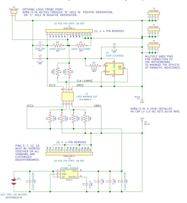
Its operation is similar to that of the standard daughterboard, except that provision has been added for a user-configurable output-side oscillator.
