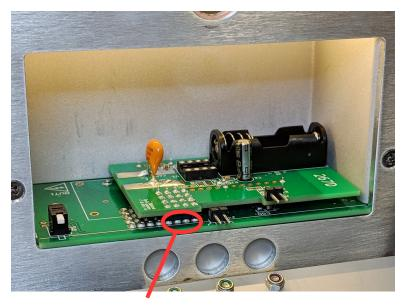
The right-most four GND2 pin sockets are used in the negative orientation.
