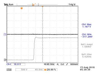
No significant logic output glitch for  $t_{R10-90}$  = 5.426 ns, so the CMTI exceeds 1.5 kV × (90%-10%) / 5.426 ns = 221 kV/us when  $I_F$  = 0 mA.
