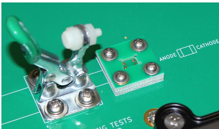
Using tweezers, position a DUT in the cavity of the raised circuit boards. The DUT will rest on four spring pins, with two contacting each DUT pad:
