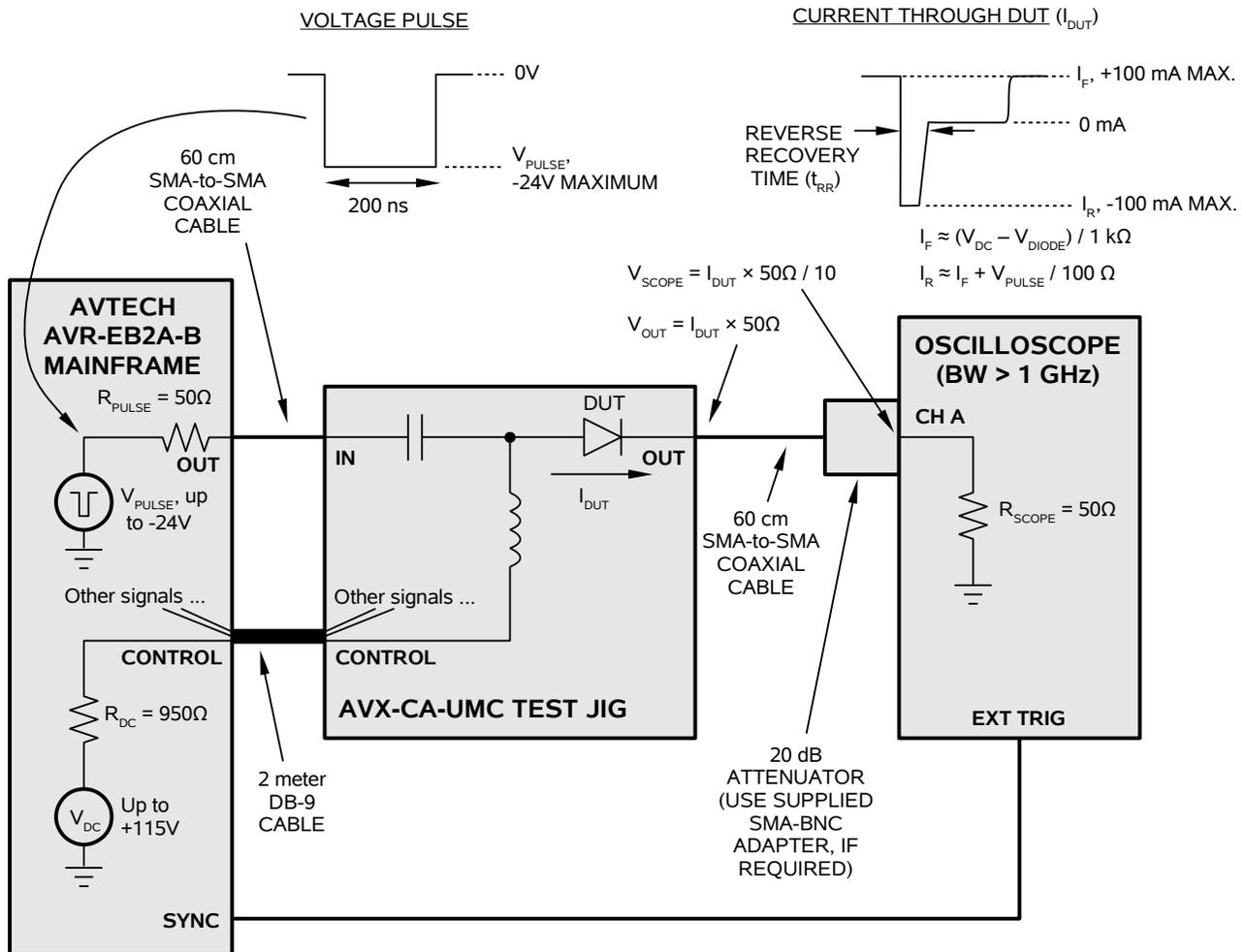
The OUT output on the test jig must be connected (using the 60 cm SMA-to-SMA cable and 20 dB attenuator supplied with the AVR-EB2A-B) to the 50 Ohm input of a high-bandwidth (> 1 GHz) user-supplied oscilloscope. The voltage on the output is proportional to the current through the DUT. By observing the current waveform
