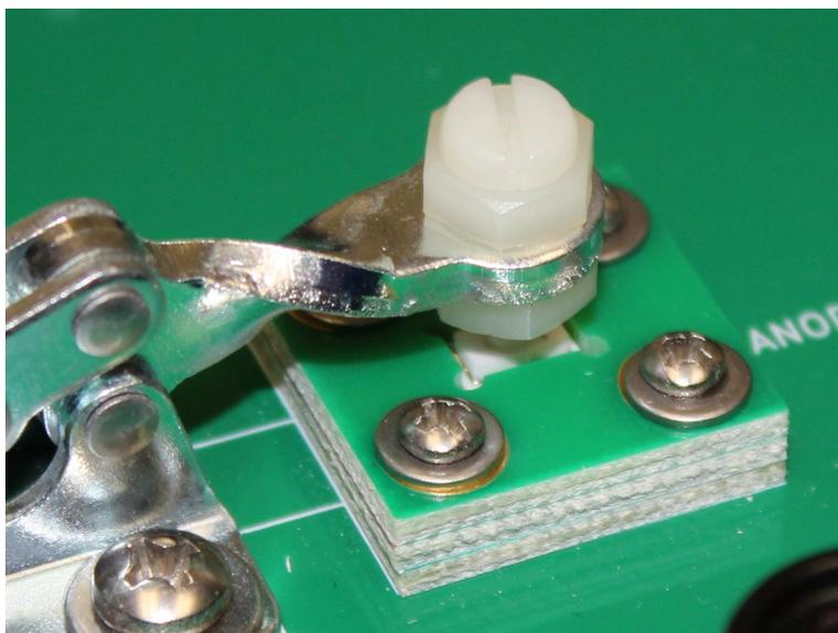
(It is possible to use a screwdriver to adjust the positioning of the nylon screw. This will vary the maximum mechanical pressure applied to the DUT.)
