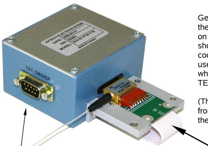
Gently slide the low-bandwidth slide-on socket onto the matching pins of the device under test. The slide-on socket is connected to the output module using a short length of flexible ribbon cable. The thermoelectric cooler and thermistor pins are made accessible to the user through the “TEC DRIVER” DB-9 connector, which will mate to cables from common third-party TEC controllers.
