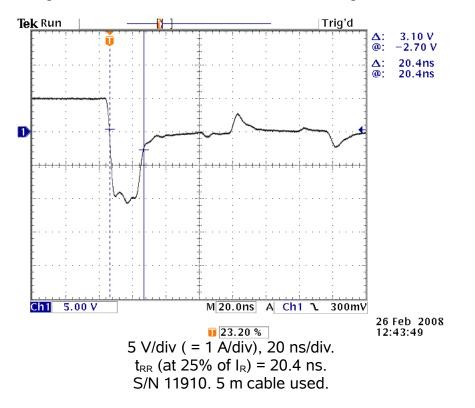
The turn-off transient of the MQ1N5811US is a classic "hard", "snap" or "step" recovery (as opposed to a "soft" recovery), causing alternating-polarity transmission line reflections (seen in the second half of the time scale above). To ensure that these reflections do not overlap with the measurement area, a 5-meter-long cable was used to connect the AVX-TRR-SQMELF to the AVR-EB4-B. See the AVR-EB4-B manual for additional details about reflections and cable length issues.
