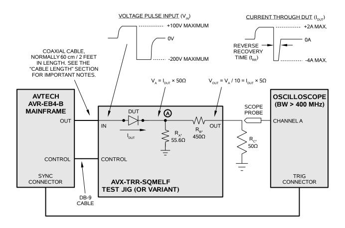
$\underline{/!}$  A 50 Ohm resistance (R<sub>c</sub> in the diagram above) must be connected to ground on the output. This can be a discrete resistor, a feed-through terminator, or the input impedance of an oscilloscope. If a high-speed sampling oscilloscope is used, the input should be protected by adding attenuator on the input.
