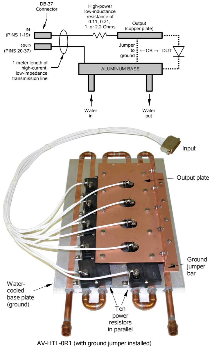
The jumper bar is installed when shipped from the factory.
